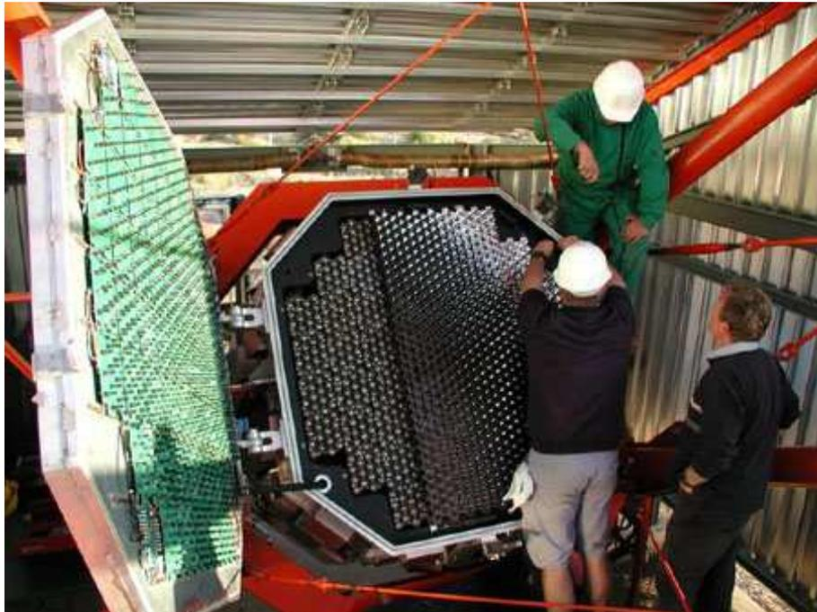
Figure 12: Top end detector for the first HESS telescope. Note the array of 960 photomultipliers.
