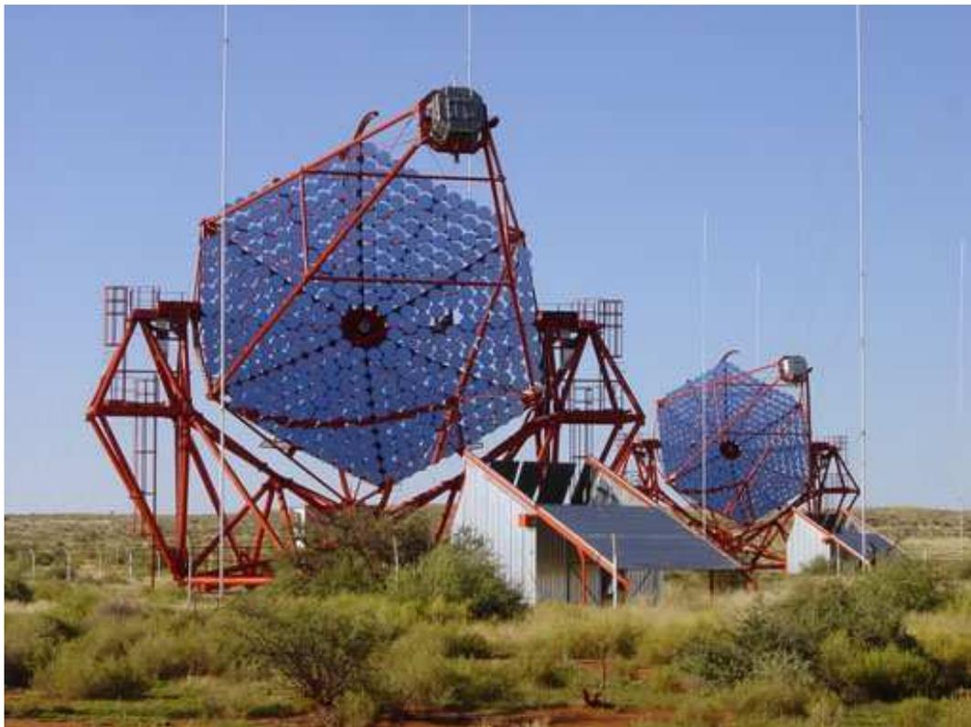
Figure 11: Two of the four (Phase 1)  $\sim 11\text{m}$  telescopes of the HESS telescopes for detecting Čerenkov radiation from high energy cosmic rays.
